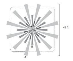
A: When walking across beam, detection will occur at approximately 22 feet.B: When walking into beam, detection will occur at approximately 12 feet.
