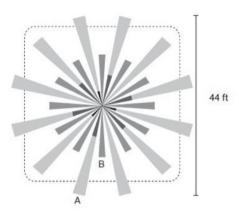
A: When walking across beam, detection will occur at approximately 22 feet. B: When walking into beam, detection will occur at approximately 12 feet.
