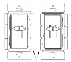
Tabs Removed for Mulitgang installation
