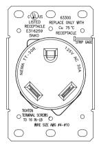
NEMA TT-30R 2 Pole, 3-Wire Grounding 30A 125 VAC, 60Hz
