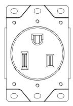
NEMA 6-50R 2 Pole, 3 Wire, Grounding Rated at 50A 250 VAC, 60Hz
