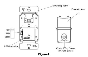
Manual ON/OFF Button: The push button may be used to manually turn ON/ OFF the load. The Load will turn ON ONLY when the push button is used and automatically turns OFF when the selected time delay has expired. If the time delay has expired and the Load turns OFF, the Load will turn ON again automatically if motion is detected within 30 seconds.
