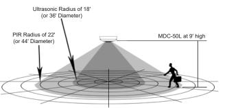
**Location:** Device should be mounted in a location free of obstruction from furniture, plants, walls and vibration (see Figure 1). The sensor must be mounted a minimum of 4 ft. away from any air vents. Avoid mounting the sensor close to heat source. When mounting directly to a ceiling light fixture, the lens of the sensor must be below the lowest point of the fixture.
