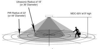
**Location:** Device should be mounted in a location free of obstruction from furniture, plants, walls and vibration (see Figure 1). The sensor must be mounted a minimum of 4 ft. away from any air vents. Avoid mounting the sensor close to heat source. When mounting directly to a ceiling light fixture, the lens of the sensor must be below the lowest point of the fixture.
