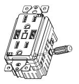
To replace the face cover, use a flat screwdriver and insert the tip at the gap shown in the diagram above and pry cover off. To re-install, simply align the cover and snap back on.
