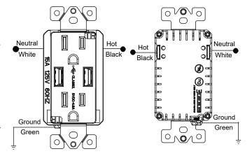
**Safe charging:** The USB ports protects your devices from over-current, over-charging, and short circuit. Depending on your device and use of quality cables, charging times may vary.
